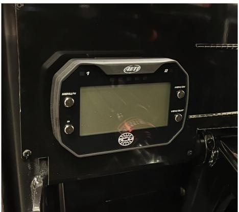
This dashboard (gauge) is intended to be used with the AIM ECU. The AIM ECU is currently being used by US Legend Cars International as a direct stock replacement for the GET ECU.
